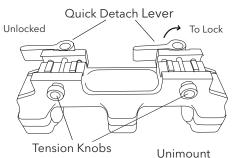
Lock by pushing down on the levers to fit securely so there is no movement. Adjust the Tension Knobs of the levers' counter bolt as needed. Do this for both levers.
